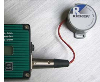
Photo C: RAS with 1 remote H4 sensor
