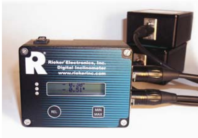
Photo A: RAD with 2 remote Nema 4 Box/Sensors
