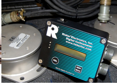
Photo B: RAD with 2 remote Subsea Sensors
