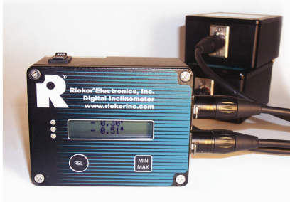
Photo A: RAD with 2 remote Nema 4 Box/Sensors
